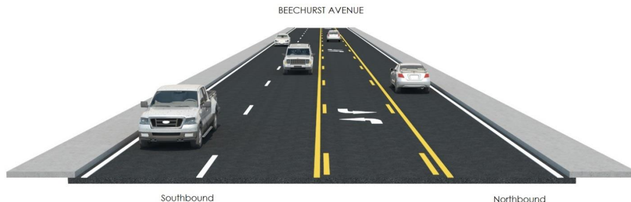
Figure 7 – Typical Section (2 Lanes SB, 1 Center 2-Way Left Turn Lane, 1 Lane NB)
